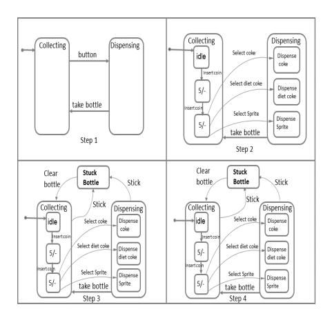
The above diagram explains the entire procedure of a bottle dispensing machine. On pressing the button after inserting coin, the machine will toggle between bottle filling and dispensing modes. When a required request bottle is available, it dispense the bottle. In the background, another procedure runs where any stuck bottle will be cleared. The 'H' symbol in Step 4, indicates that a procedure is added to History for future access.
